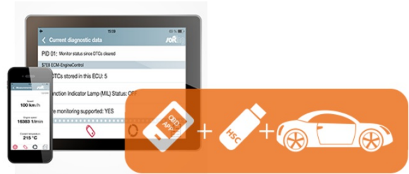
With the OBD app the user can read all in-vehicle diagnostic data on their smartphone or tablet computer (Photo: Softing)
