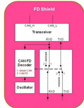
Block diagram of the CAN FD Shield transceiver (Photo: NXP)
