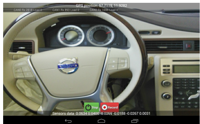
The simulation environment can monitor up to 8 CAN channels (Photo: Zuragon)
