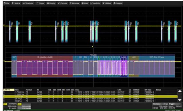
CAN FD TDM provides flexible triggering for CAN and CAN FD data, error, and remote frames (Photo: Teledyne LeCroy)
