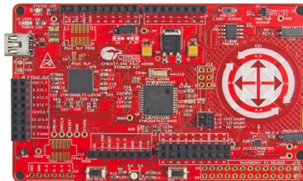
The Pioneer Kit features the PSoC 4200M device with CAN peripherals (Photo: Cypress)
