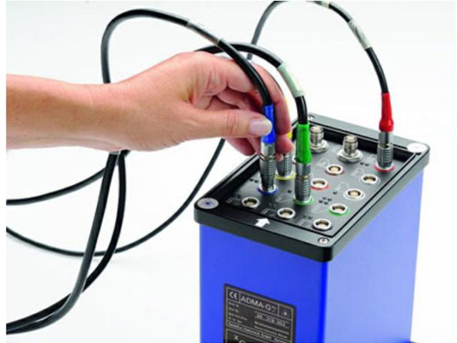
Adma with an output rate of 1000 Hz (Photo: Genesys)
