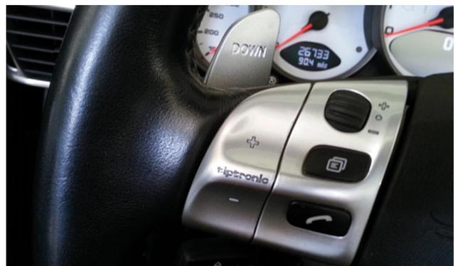
*The system is connected to the factory installed steering wheel remote control via a CAN interface (Photo: Zenec)*
