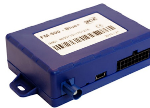
The gateway complies with the FMS specification based on the J1939 application layer (Photo: BCE)
