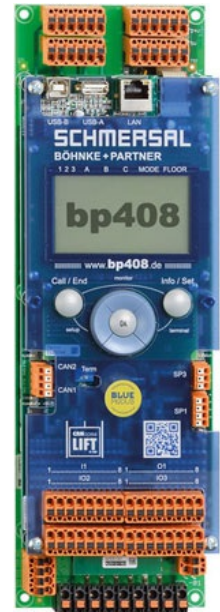
The lift controller module can even be fitted into doorframes (Photo: Schmersal)
