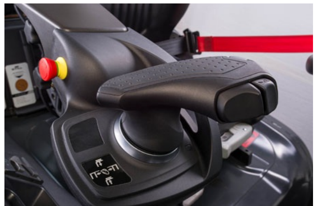
Like the previous model, the redesigned joystick contains a rocker for driving direction and tilt, the lateral movement of the forks, as well as an additional function key and a horn button (Photo: Still / Elobau)
