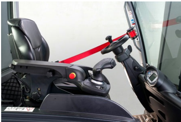
With its reach and counterbalance trucks, Still offers a cockpit which includes an Elobau multifunction control (Photo: Still / Elobau)
