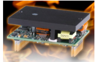
The DZX series with CANopen servo drives (Photo: Advanced Motion Controls)
