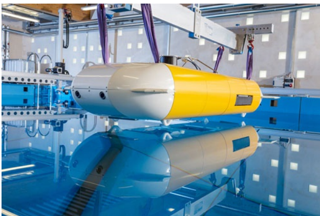
The AUV weighs less than 700 kg, making it a lightweight vehicle (Photo: Fraunhofer IOSB-AST)
