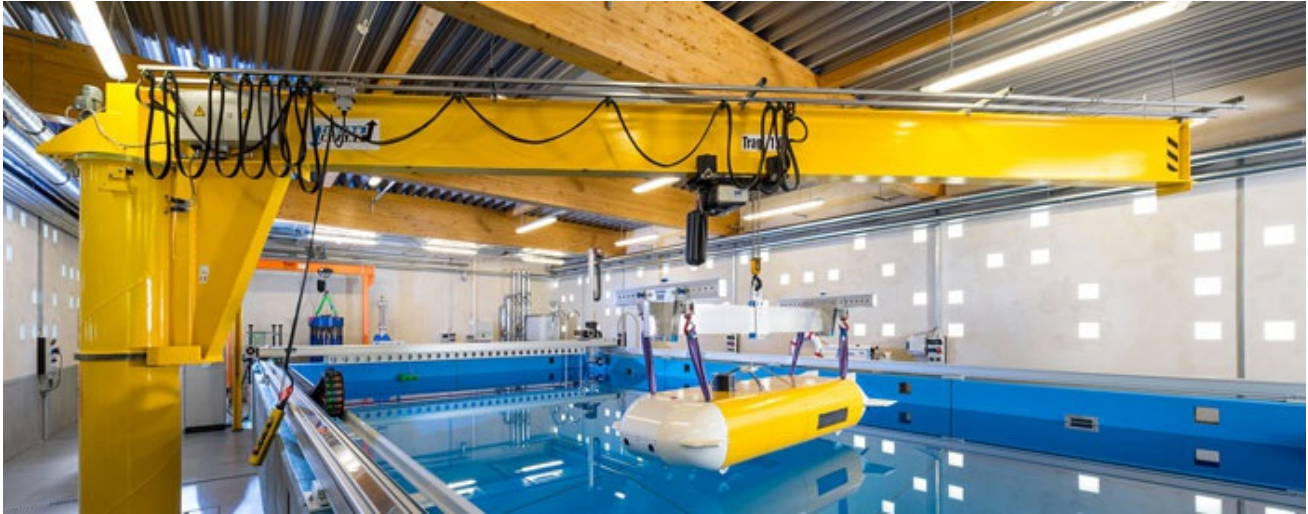
The underwater vehicle suspended above the maritime systems research platform with its slewing crane, portal system and (in the background on the left) pressure chamber (Photo: Fraunhofer IOSB-AST)
