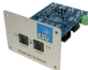
The ECoSlink terminal provides a CAN interface and is used for Pullman model railroads (Photo: ESU)
