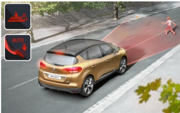
The Renault Scenic shown at the Motorshow in Geneva monitors the vehicle environment, alerts the driver to collision risks, and triggers the brakes automatically if necessary; other ADAS features include lane keeping and fatigue detection systems (Photo: Renault)
