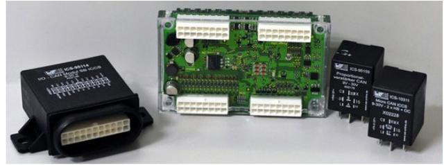
From left to right: The CAN I/O, the CAN Controller 64P, the PropCAN, and the Micro CAN modules (Photo: Wuerth Elektronik)
