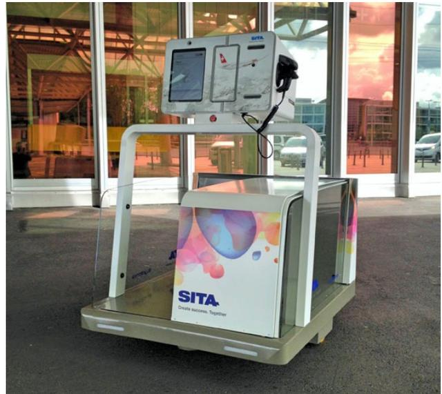
Leo is an autonomous baggage robot that can check in, print bag tags, and transport up to two bags (Photo: Bluebotics)
