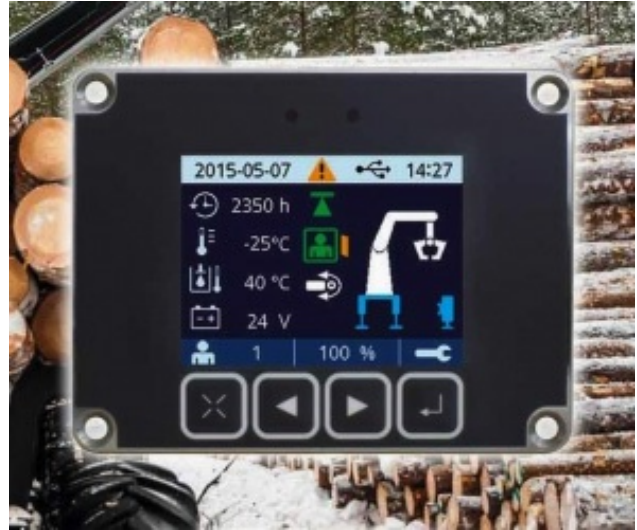
xCrane can be connected with the tractor via J1939 (Photo: Kronos)
