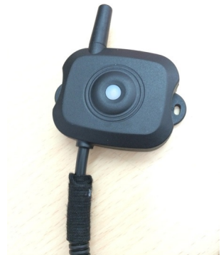
The CAN module measures 84 mm x 58 mm x 34 mm and has IP65 (Photo: Tyrepal)
