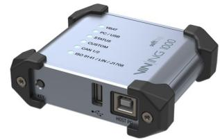
*The Vining 1000 has an operating temperature of -40 °C to +70 °C
