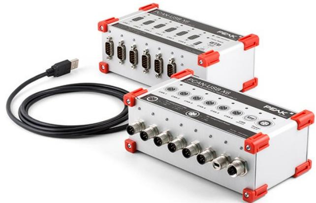
*PCAN-USB X6 with M12 circular connectors is expected to be available in Q4 2016 (Photo: Peak-System)*
