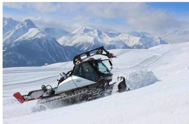
*The Leitwolf is the world's first production vehicle in its class to meet the "Stage IV/Tier 4 final" exhaust emission standard (Photo: Prinoth)*
