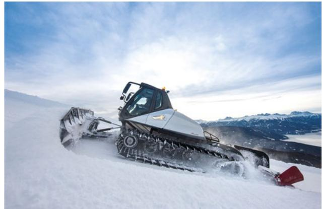
*The snow groomer Leitwolf is the strongest vehicle of its class: the six-cylinder diesel engine has an output of 390 kW and generates torque of 2460 Nm (Photo: Prinoth)*
