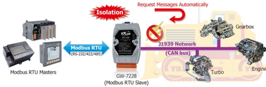
Block diagram of a connection between a CAN-based J1939 network and a Modbus-RTU controller (Photo: ICP DAS)
