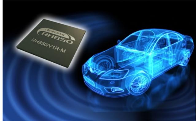
*The RH850/V1R-M dual-core micro-controller has six CAN FD ports
