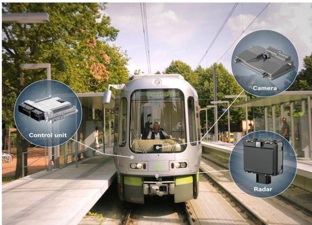
*The system combines a radar sensor with a video sensor to detect any cars, buses, nearby rail vehicles, and static obstacles on the tracks (Photo: Bosch)*
