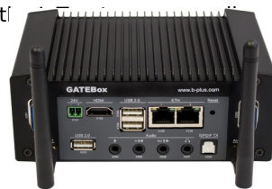
The Gatebox 100 LTE gateway links the in-vehicle networks to the cloud (Photo: B-Plus)
