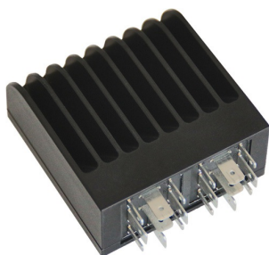
The b-CANCubeMini control unit is suitable for vehicle body applications (Photo: B-Plus)
