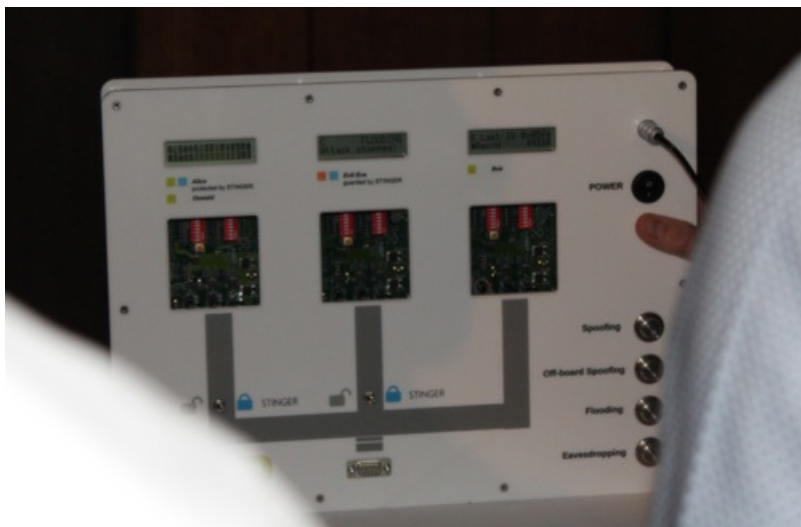
Demonstrator of the secure CAN FD transceivers qualified for 5 Mbit/s (Photo: CiA)
