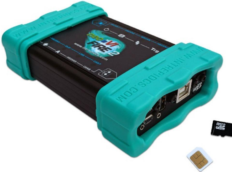
The NeoVI Fire 2 module can be connected via USB to PCs or be operated as a stand-alone device (Photo: Intrepid)
