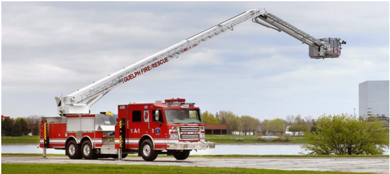
The T-Rex articulating platform mounted on a fire-fighting truck (Photo: Rosenbauer)
