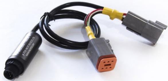
The CAN Engine Gateway YDEG-04 dongle links CAN networks to USB (Photo: Yacht Devices)
