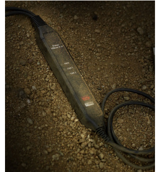
The CAN interface modules feature galvanic isolation (Photo: Kvaser)
