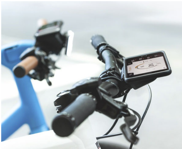
The smartphone hub provides a CAN interface (Photo: Cobi)
