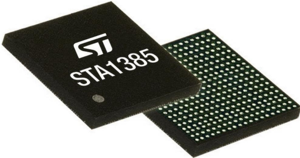
STA1385 is an automotive, System-on-Chip, targeting processing solutions for telematics and connectivity applications including cyber-security protection (Photo: STMicroelectronics)
