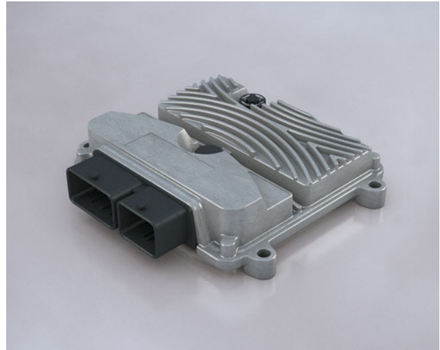
The controllers come with six CAN interfaces (Photo: STW)
