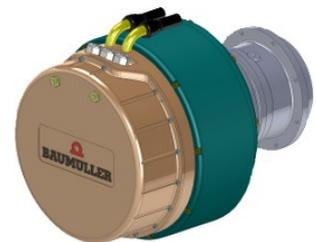
*The electric axle consists of a DSA synchronous external rotor motor with planetary gear and integrated line electronics with motor controller and converter (Photo: Baumüller)*
