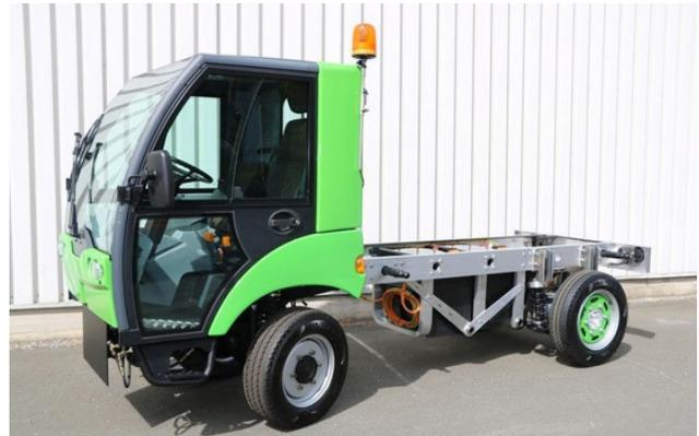
*The municipal vehicle developed jointly in a research project is intended for series production and can achieve ranges up to 100 km (Photo: Baumüller)*
