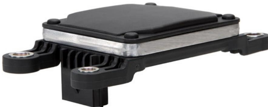
With long-range radar, a range of up to 300 m and an opening angle of  $\pm 60^\circ$  are possible in the highest expansion stage depending on the required performance (Photo: Continental)
