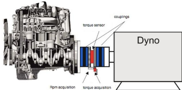
Integration in a test stand (Photo: Manner Sensortelemetrie)
