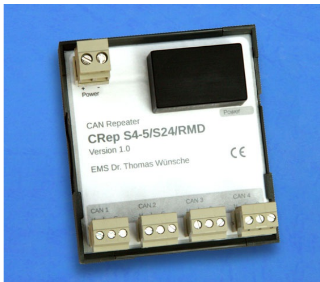
The CRep S4 star repeater (Photo: EMS Wuensche)
