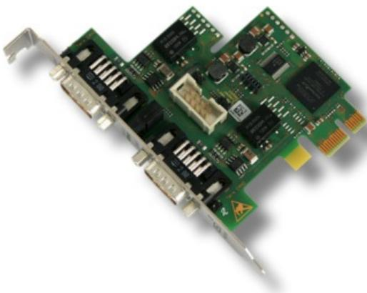
Sometimes, you need to dig deeper, in order to see CAN-based products such as the PCI interface board used in the Baidu Apollo reference hardware platform (Photo: ESD)
