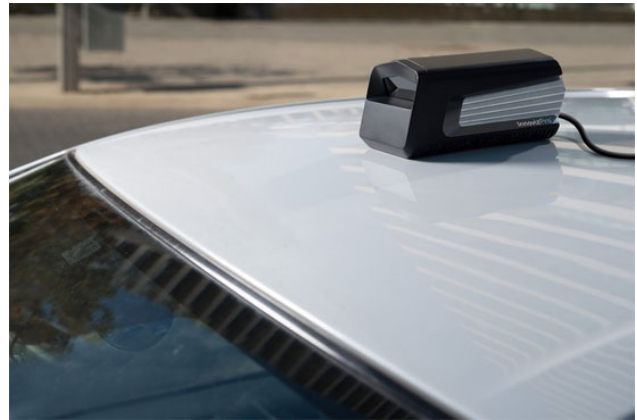
The solid-state lidar features a detection range of up to 150 m (Photo: Innoviz)
