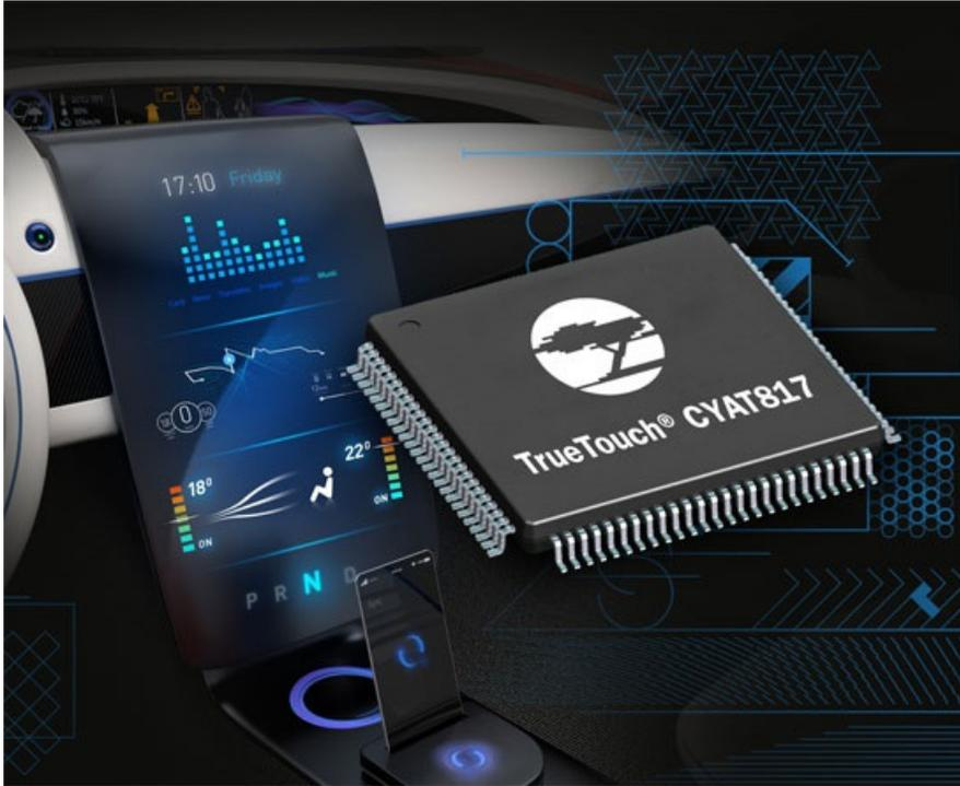
The CYAT817 supports two standard host interfaces such as I<sup>2</sup>C and SPI as host interfaces, along with a CAN interface for either higher system integration or to implement redundancy for safety relevant applications per ISO 26262 (Photo: Cypress)
