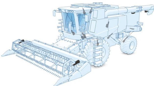
*Linear electromechanical drives are suitable for "machines on wheels" such as agriculture off-highway vehicles (Photo: Thomson)*
