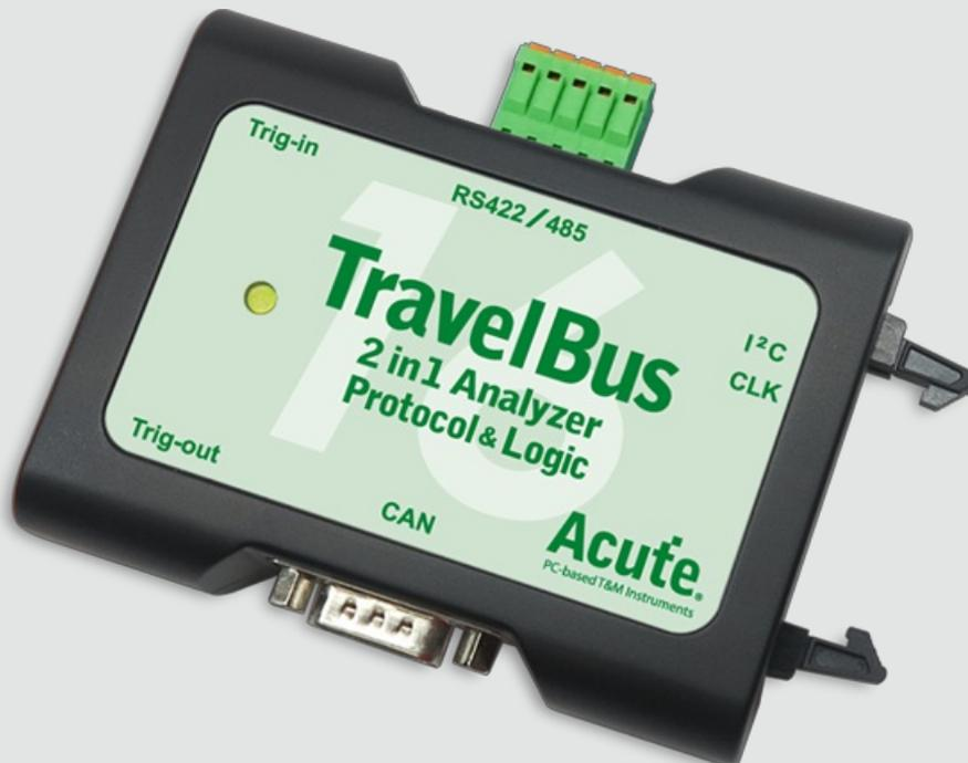
The Travelbus module records the CAN traffic and forwards the data to the PC for analyzing it (Photo: Acute)
