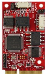
The termination resistors for the two CAN channels can be enabled and disabled by means of jumper (Photo: Innodisk)
