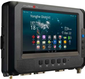
*The CAN connectivity supports the OBDII protocols as well as SAE J1939 communication (Photo: Ruggon)*
