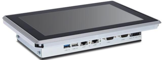
*Besides CAN, interfaces such as Ethernet, USB, and EIA-232 are also options (Photo: Syslogic)*
