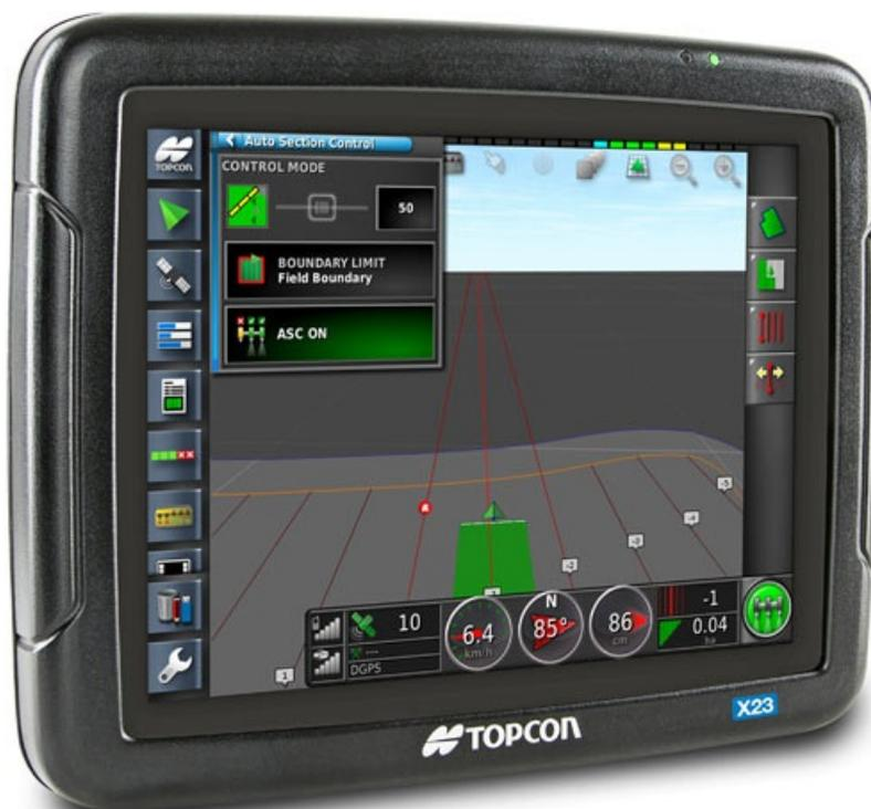
The X23 offers functions such as variable rate application and auto-section control; each icon-based screen can be configured to create a user-defined implement control system (Photo: LH Agro)
