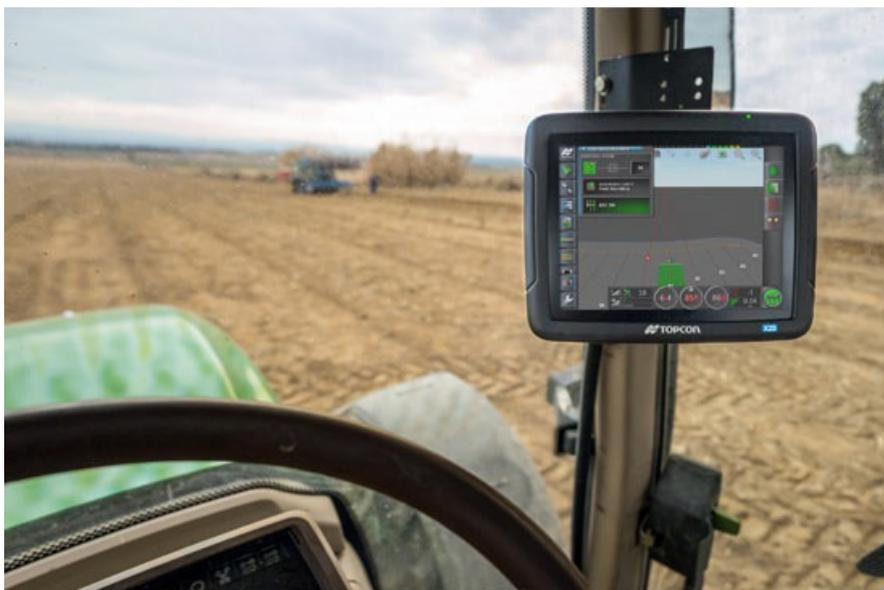
Compatible with all makes and models of tractors, sprayers, combine harvesters, and Isobus implements, the X23 is Topcon's entry-level precision farming control console (Photo: LH Agro)
