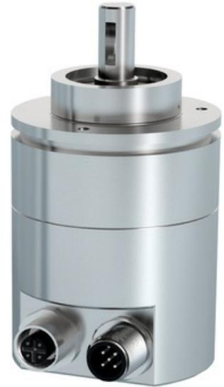
*The TBN58 Class-2 encoder comes with a CANopen interface compliant to CiA 406 version 4.0.1 (Photo: TWK)*
