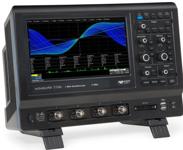
Add-on software enables the oscilloscopes to analyze serial data including Classical CAN and CAN FD frames (Photo: Teledyne Lecroy)
