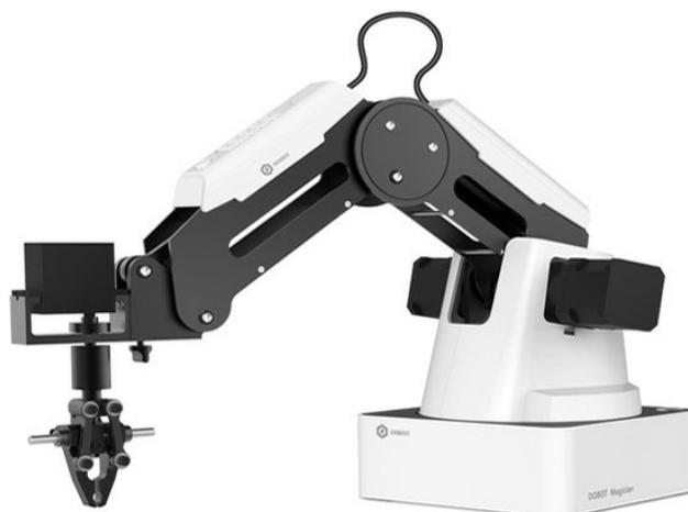
The Dobot Magician is a 4-axes robot system providing a CAN interface (Photo: Variobotic)
