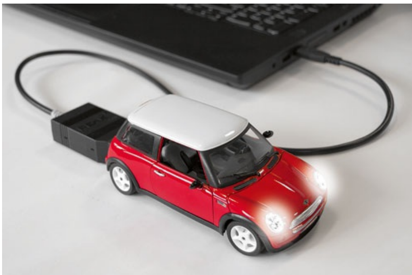
The adapter provided by Peak comes with CAN FD and LIN interfaces (Photo: Kithara)
